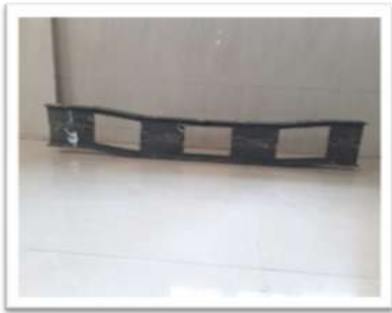
Figure. 3 Web and flange buckling is observed in beam with rectangular opening.
