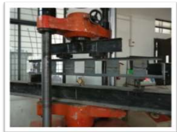
Figure. 2 Testing of Castellated beams on UTM.
